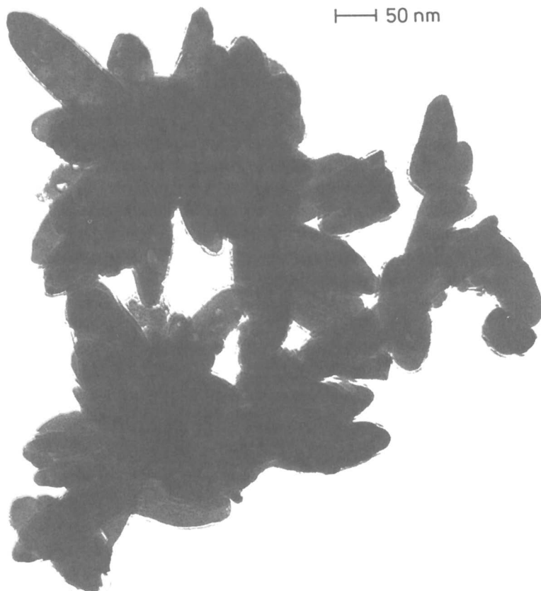
Figure 2. Transmission electron micrograph of dense-silica-coated titania particles: magnification, 200,000; 5.0 wt % silica loading. (Reproduced with permission from reference 23. Copyright 1979.)
