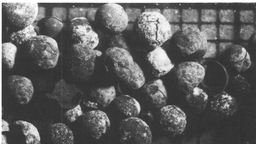
Figure 7. Effect of mercury intrusion on silica spheres (Shell). Top, starting material; and bottom, material after mercury intrusion (no attempt was made to remove the mercury).
